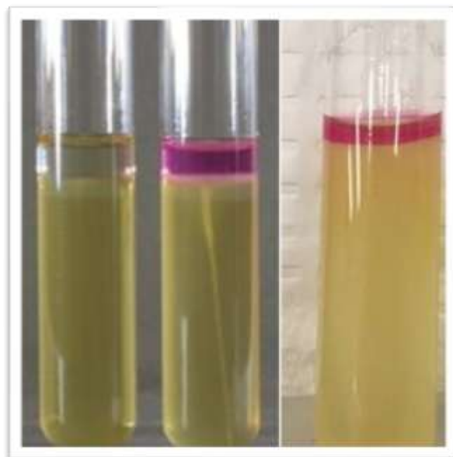
Figure 8 The pink ring indicated positive indole test results while the brown ring indicated no indole production.
